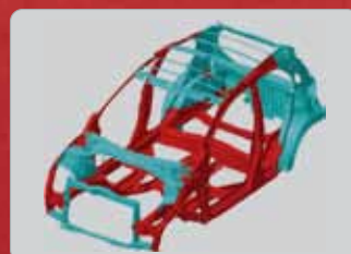
ACE™ Body disperses and absorbs collision impact
