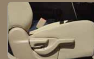
NEW Seat height adjuster that helps you find a comfortable seating position
